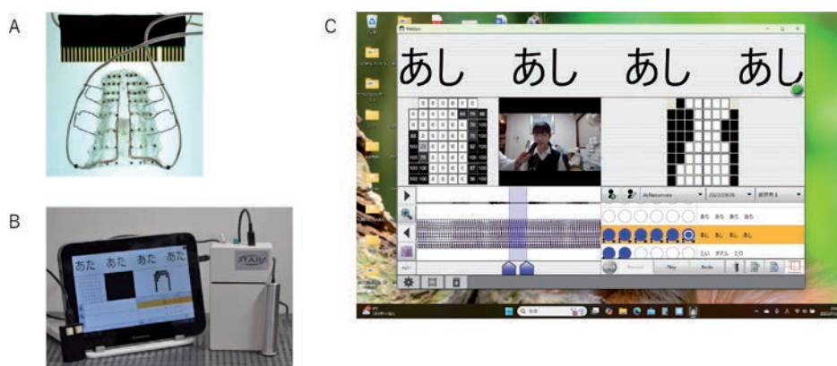
Figure 1. EPG equipment. A: EPG artificial plate (McYam Plate) B: EPG system (WinSTARS). C: Screenshot of WinSTARS.
